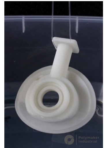
Figure 4. Dip the PolyCast™ pattern into isopropyl alcohol
