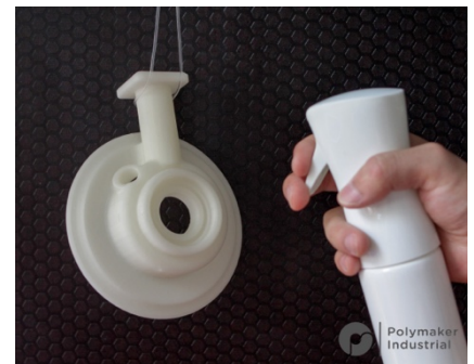
Figure 5. Spray isopropyl alcohol on the PolyCast™ pattern
