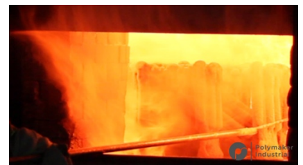
Figure 8. Sinter the ceramic shell and burnout
