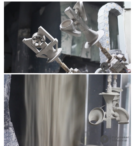
Figure 7. Make the ceramic shell
