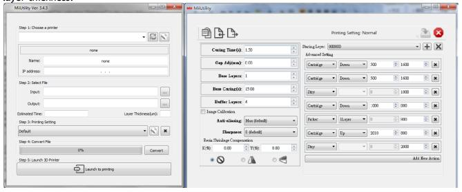
The last step is to modify the printers LED power. This can be done by entering the machine's IP-address in your browser or by clicking "Launch to printing" in the window above. The window below will appear.
